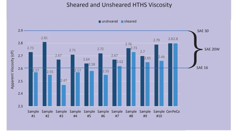
viscosity was tested. Six of the ten samples failed to meet the 2.6 cP minimum requirement—all of the conventional oils and one of the synthetic oils.
